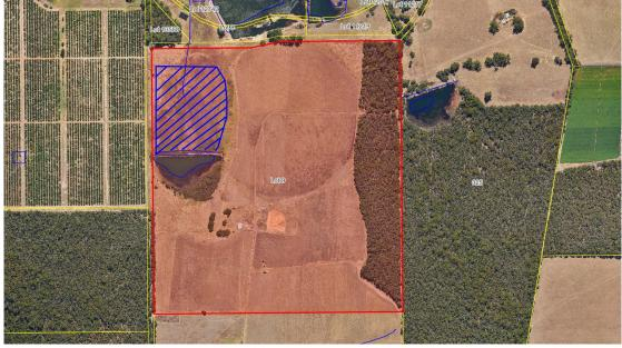
Plans and details submitted with the application indicate that the dam wall facing the front boundary, will have a whole crest length of 628m running north south along the side boundary for approximately 360m before it projects approximately 268m east along the northern boundary.
