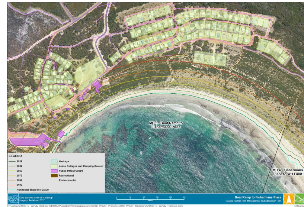
Figure 3-2 Projected Erosion Hazard Lines for MU3
